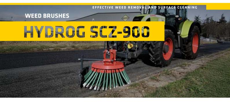
The **HYDROG SCZ-900** is a professional weed brush system designed for mechanical removal of weeds and debris from paving stones, sidewalks, concrete block surfaces, and other hardened surfaces. With its powerful and efficient brushes, it effectively eliminates overgrown plants without the use of chemicals, making it an eco-friendly and safe solution for municipalities and maintenance companies.
