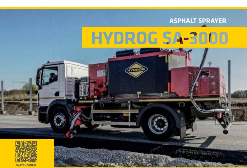
Capacity of 3,000 liters, equipped with an oil-jacket **Asphalt Tank Operating Temperature** of Asphalt **Heating Burner Type Asphalt Mixing** Hydraulically driven vertical agitator **Asphalt Filling** using the machine's own pump (suction function) **Diesel Engine Asphalt Pump** Positioned in front of the vehicle's axle Main Working Hydraulically extendable and tiltable Component - Side **Spraying Ramp** Adjustability of Side Ramp Position
