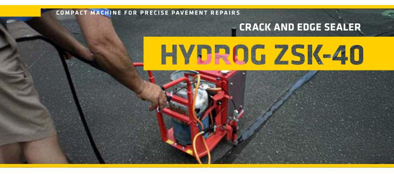
The **HYDROG ZSK-40** is a mobile and easy-to-use crack and edge sealer, ideal for quick and effective road surface repairs. Thanks to its compact size and simple design, it can be operated by a single operator, minimizing labor costs and increasing operational efficiency.
