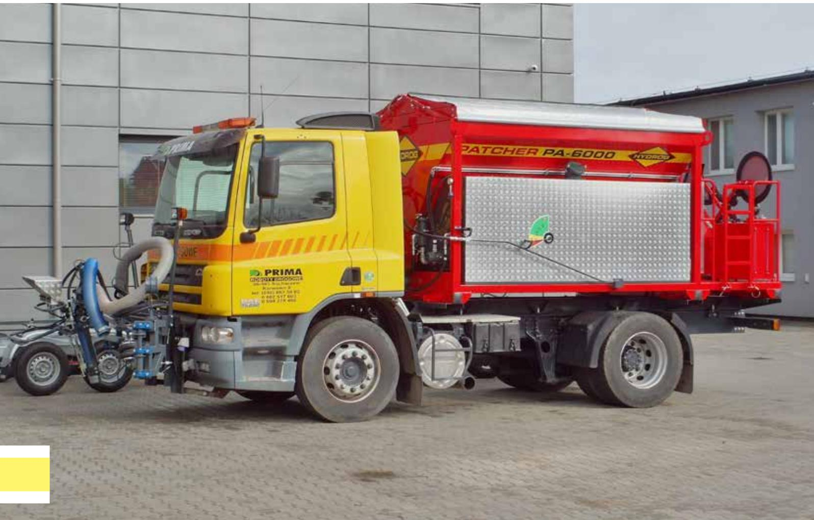
Blow patcher Hydrog PA-5000 / PA-5000 is intended for repair of bituminous surfaces by filling and sealing potholes with mineral aggregate coated by bitumen emulsion. The aggregate is fed in a stream of air generated by a blower through a flexible hose to the working head, in which it is coated with bitumen emulsion.
