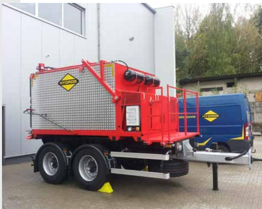
Thanks to the speed control, the operator can optimise the performance of the auger feeder. The largest loading hole on the market enables asphalt concrete to be loaded in every asphalt plant,
