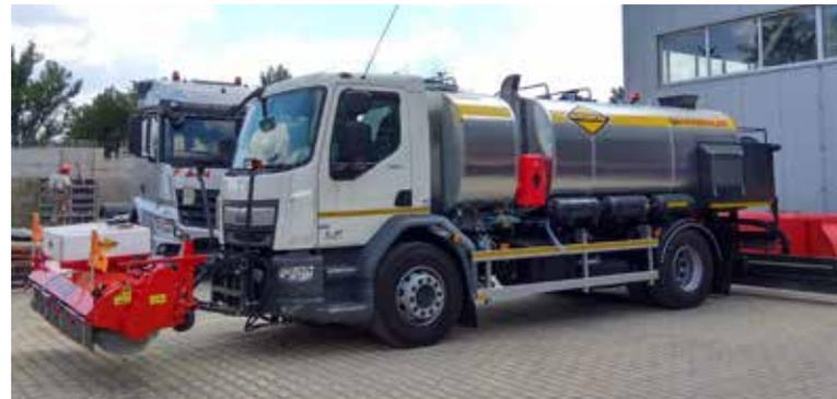
**Unique on the market, innovative solutions make SH PREMIUM class sprayers more environmentally friendly and economical. For example, when heating a full emulsion tank, the burner will consume about 10 litres less oil than other brands of machines. After spraying, the machine will automatically clean the pump and spray bars from emulsion residues.**
